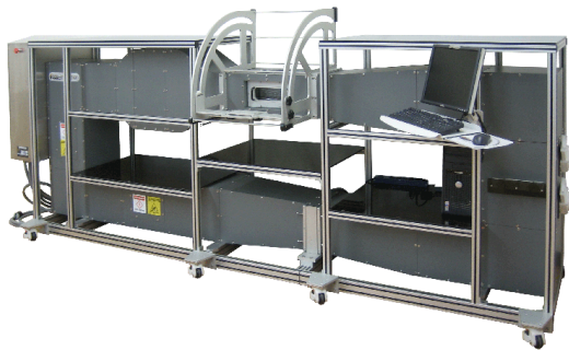
Fig. F: FDK Original Wind Tunnel
