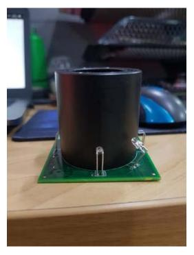
The test vial should be screwed into the EVAL-CN0409-ARDZ board, by lining up the holes in the vial holder with the holes in the board, using the screws provided.
