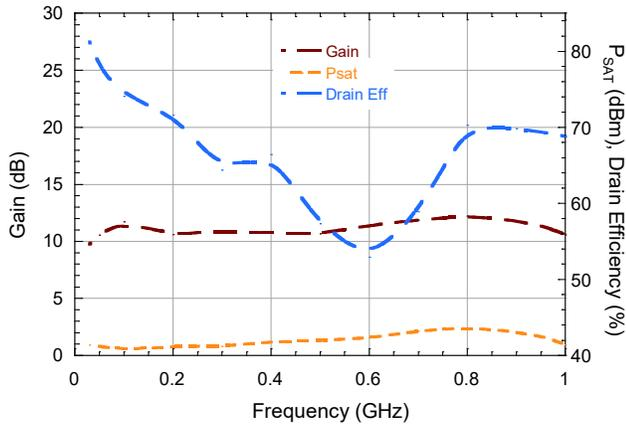
Performance vs. Frequency at  $P_{OUT} = 41\text{ dBm}$
