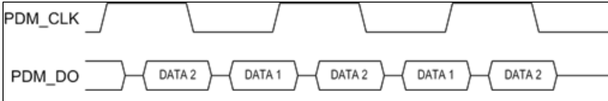
Figure 7 PDM Two-Channel Output Timing
