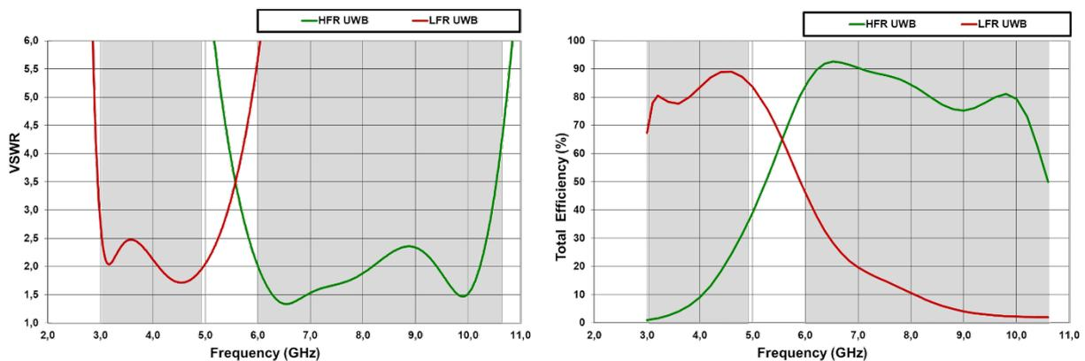
**Figure 4** – VSWR and total efficiency for the UWB LFR (3.1GHz – 4.8GHz) and for the UWB HFR (6.0GHz – 10.6GHz) from the Evaluation Board (Figure 1 with the matching networks gathered in Figure 2 (LFR UWB) and Figure 3 (HFR UWB), respectively. Simulated results obtained with CST.
