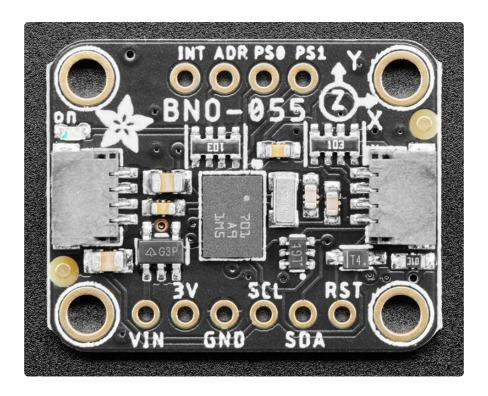
Note: The pin order on the STEMMA QT version of the board is not the same as the original version. The pins are the same otherwise.
