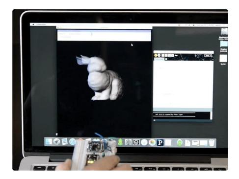
Also notice in the upper right corner of the dialog box at the top that the calibration of each sensor is displayed. It's important to calibrate the BNO055 sensor so that the most accurate readings are retrieved. Each sensor on the board has a separate calibration status from 0 (uncalibrated) up to 3 (fully calibrated). Check out the <a href="video">video</a> and information from this guide for how to best calibrate the BNO055 sensor ().
