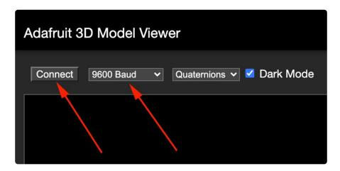
When the security window pops up, pick the matching Serial/COM port for your board running the AHRS sketches. Make sure the serial port isn't open in Arduino or something else.
