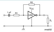
Maximum  $V_{o(p-p)} = V_{CC} - 1.5 \text{ V}$  centered at  $0.5 \times V_{CC}$ .
