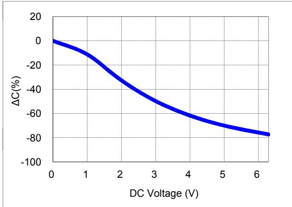
4) Bias TCC characteristics (Agilent 4284A, 120Hz, 0.5Vrms, 3.15Vdc)
