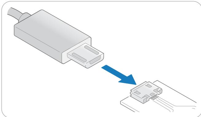
4. Make sure no object is within the touch active area of the sensor module before connecting power to the sensor through USB. The sensor calibrates itself when powered on and an object within the touch active area may interfere with the calibration.
