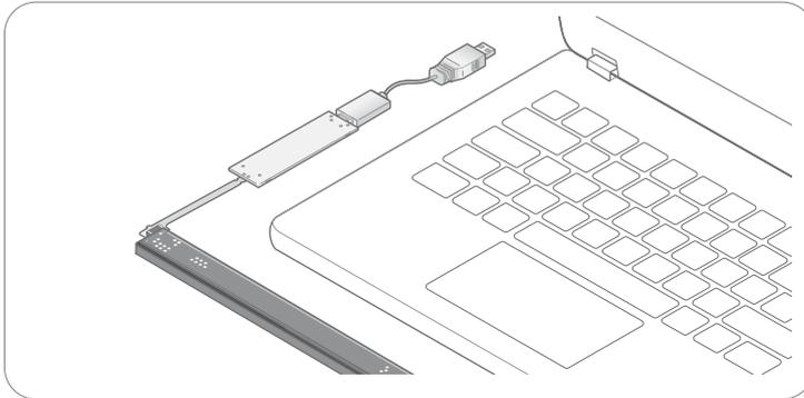
If the sensor module is of the 90° type: place the module on a table with the steel surface facing upwards, so the optical surface is facing upwards as well. Make sure no object is within the touch active area above the sensor module.
