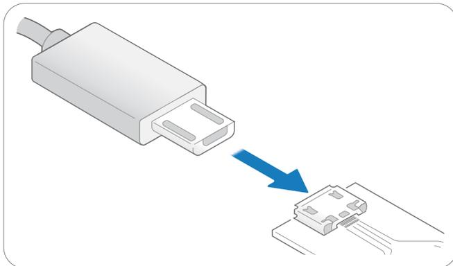
4. Make sure no object is within the touch active area of the sensor module before connecting power through USB. The sensor module calibrates itself when powered on and an object within the touch active area may interfere with the calibration.
