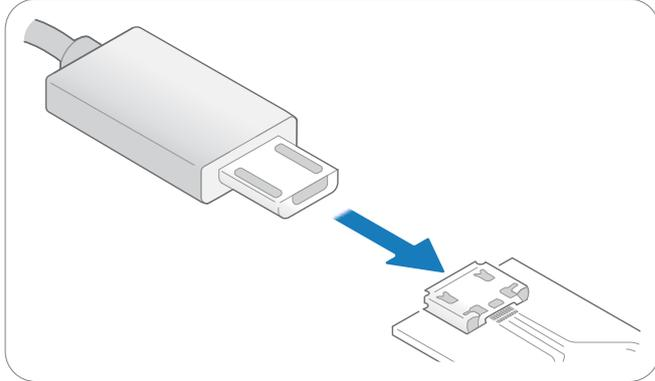
Make sure no object is within the touch active area of the sensor module before connecting power to the sensor through USB. The sensor calibrates itself when powered on and an object within the touch active area may interfere with the calibration.
