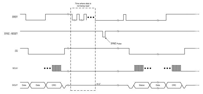
Figure 8-22. Collecting Data After a Pause in Data Collection Using the SYNC/RESET Pin
