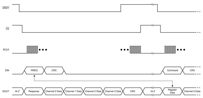
Figure 8-19. Reading a Single Register
