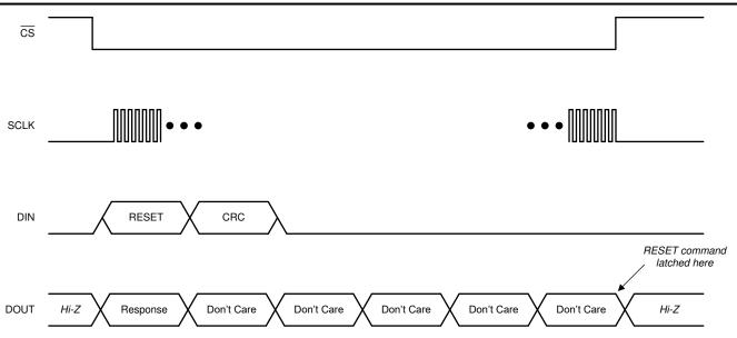
Figure 8-18. RESET Command Frame
