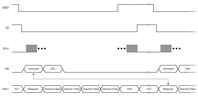
Figure 8-13. Typical Communication Frame
