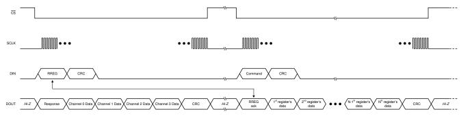
Figure 8-20. Reading Multiple Registers
