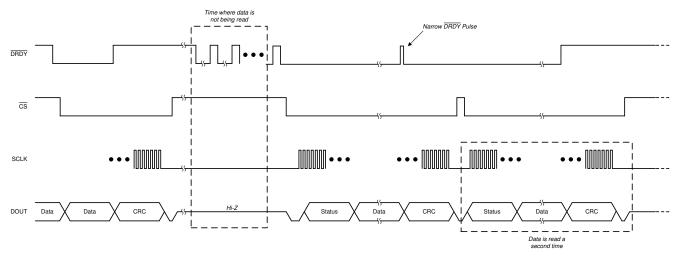
Figure 8-23. Collecting Data After a Pause in Data Collection by Reading Data Twice
