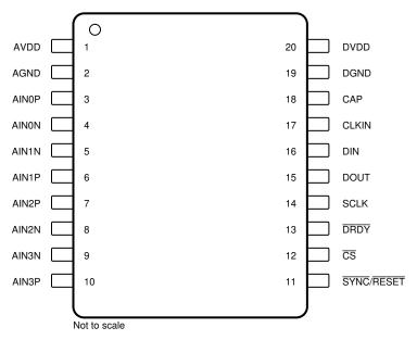
Figure 5-1. PW Package, 20-Pin TSSOP (Top View)
