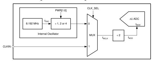
Figure 8-3. Main Clock Selection Diagram
