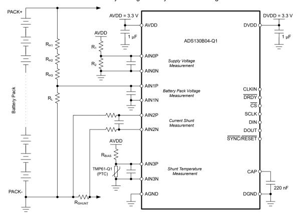
Figure 9-4. ADS130B04-Q1 in a Typical Battery Management System Application
