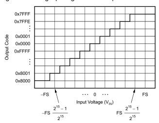
Figure 8-17. Code Transition Diagram
