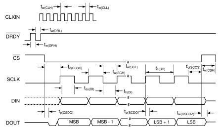
SPI settings are CPOL = 0 and CPHA = 1.  $\overline{\text{CS}}$  transitions must take place when SCLK is low.
