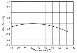
Figure 9-6. Gain Error vs Temperature
