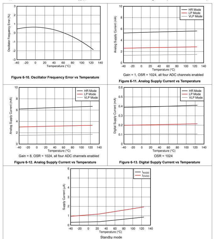
Figure 6-14. Supply Current vs Temperature
