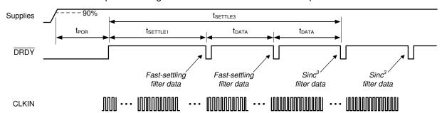
Figure 8-10. Fast Start-Up Behavior and Settling Times
