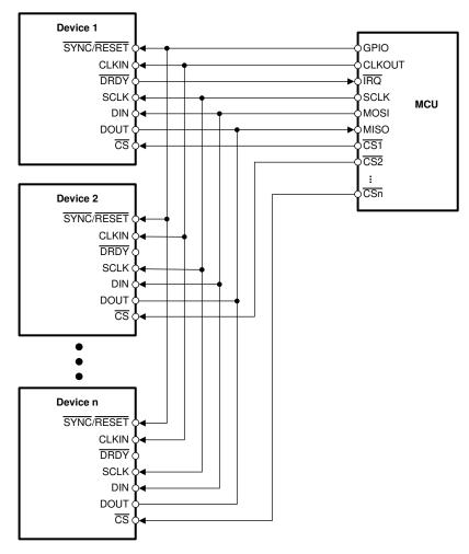
Figure 9-3. Multiple Device Configuration
