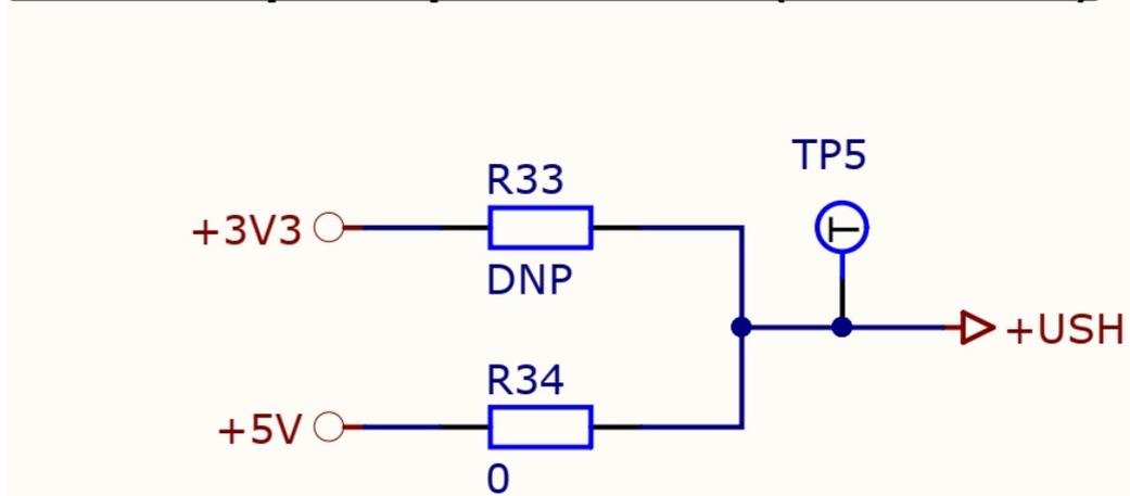
Figure 3: Power supply select for shunt amplifiers
