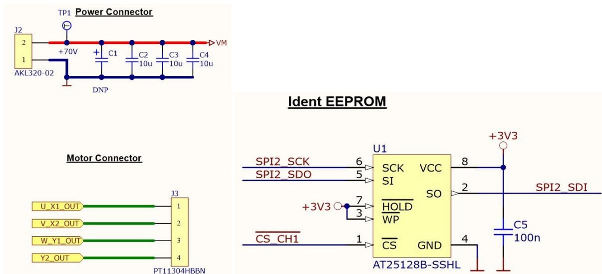
Figure 2: Motor connector, power connector and EEPROM
