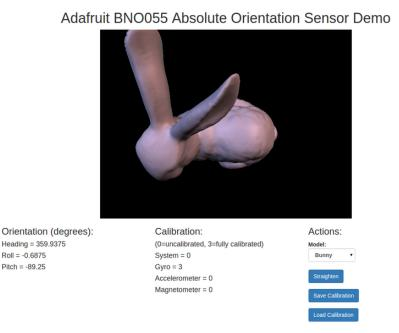
If you move the BNO055 sensor you should see the 3D model move too. However when the demo first runs the sensor will be uncalibrated and likely not providing good orientation data. Follow the next section to learn how to calibrate the sensor.
