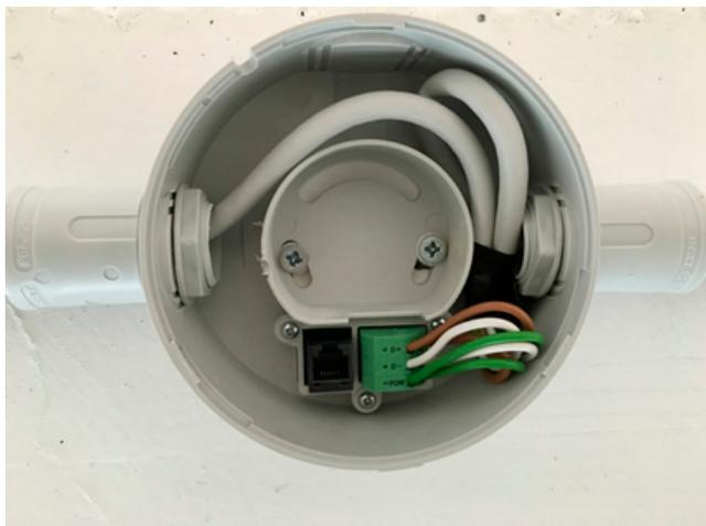
Place the wire around the inner part of the base to avoid damage of the isolation of the cable.
