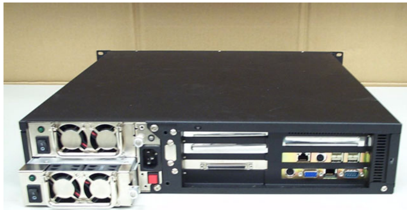
Figure 3.6 Replacing the redundant power module
