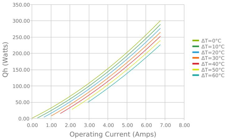
Total Heat Dissipated at Hot Side (Qh=Qc+Pin)
