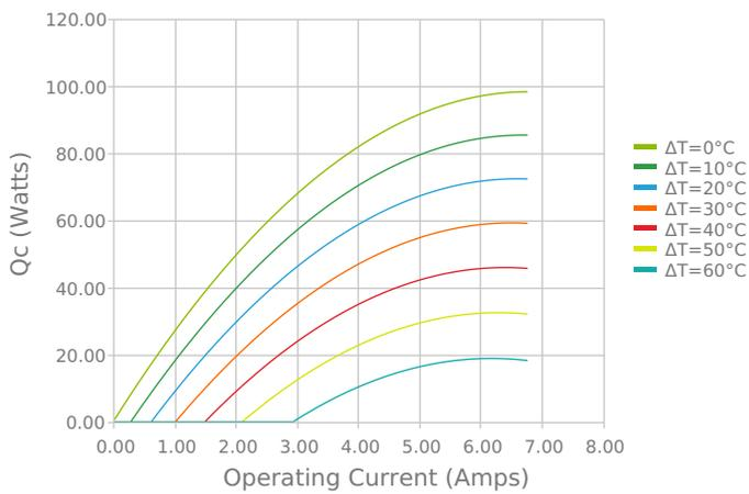
Heat Pumped at Cold Side
