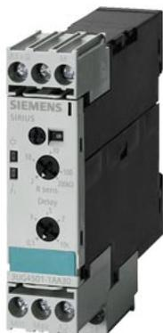
Analog monitoring relay Fill level monitoring Resistance monitoring from 2 to 200 kohm Overshoot and undershoot 24 to 240 V AC/DC 50 to 60 Hz DC and AC 2-step or 1-step control Tripping delay 0.5 to 10 s 1 change-over contact screw terminal Successor product for 3UG3501
