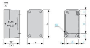
(2) 2 x Ø 5.6 mm/0.22 in. holes, depth 12 mm/0.47 in. P Usable depth
