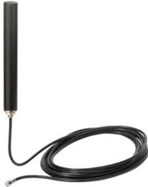
ANT794-4MR mobile wireless antenna for 2G/3G/4G EU, GSM/UMTS/ LTE EU networks, Rod antenna; omnidirectional; weatherproof for indoors and outdoors; 5 m Connection cable permanently connected to the antenna; SMA connector; incl. mounting bracket, screws, screw anchor.
