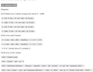
Joystick calibration method. First I2c writes register 0x03 and then sends 0x02, the joystick is rotated several times around the top, bottom, left and right, and then 0x03 is saved in register 0x03.
