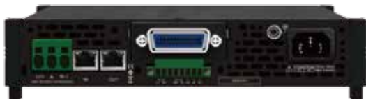
Rear panel with optional interface IT-E1208
