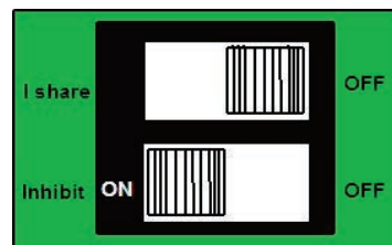
DIP Switch for Current Share & Inhibit/Enable for powerMods XgG to XgL and Xg1 to Xg5
