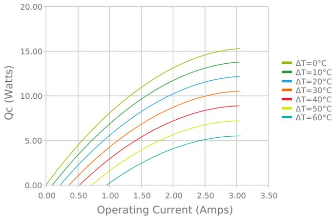
Heat Pumped at Cold Side
