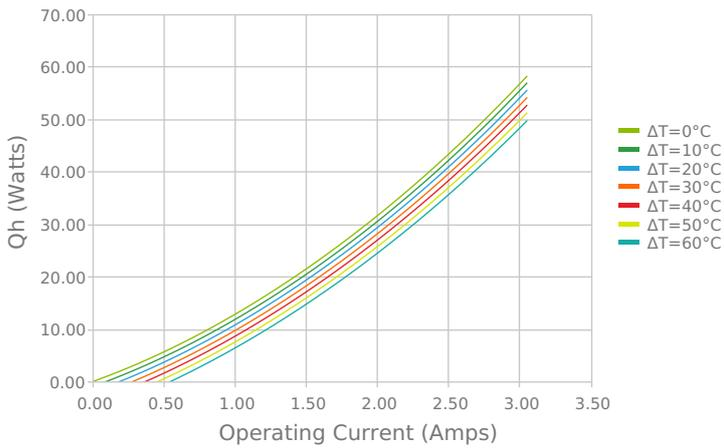
Total Heat Dissipated at Hot Side (Qh=Qc+Pin)
