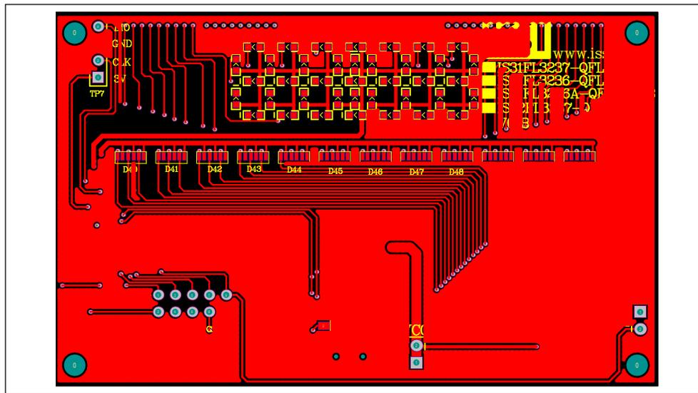
Figure 5: Board PCB Layout - Top Layer
