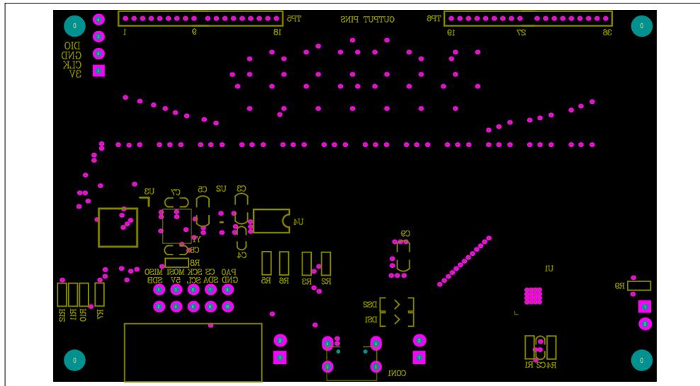
**Figure 6: Board Component Placement Guide - Bottom Layer**
