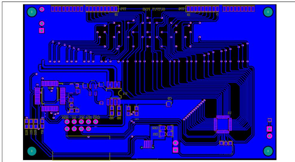
**Figure 7: Board PCB Layout - Bottom Layer**
