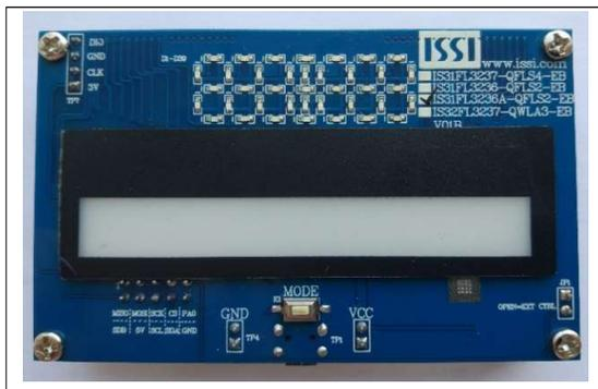
Figure 1: Photo of IS31FL3236A Evaluation Board
