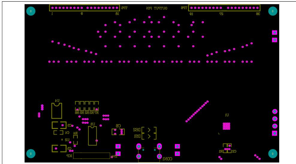
**Figure 13: Board Component Placement Guide - Bottom Layer**
