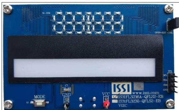
Figure 8: Photo of IS31FL3236A Evaluation Board
