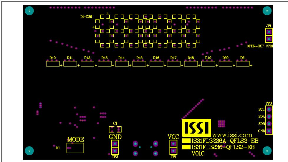
Figure 11: Board Component Placement Guide - Top Layer
