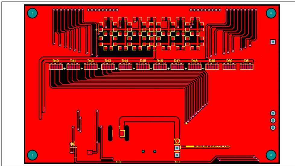
Figure 12: Board PCB Layout - Top Layer
