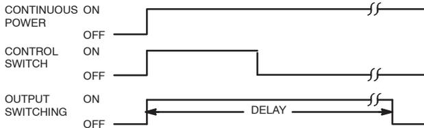
**INTERVAL ON**– The relay energizes and timing begins when the input voltage is applied. At the end of the time delay period the relay will de-energize. Reset is accomplished by removing, then reapplying the input voltage.
