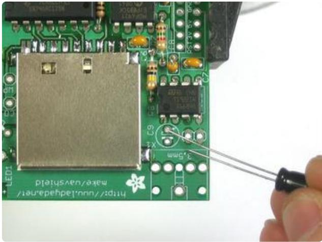
Electrolytic capacitors are polarized so make sure they go in the right way! The long lead is the positive lead, make sure that goes into the hole marked with a + as shown here.
