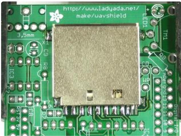
Check that you have no solder bridges - the pins should not be soldered to the metal body of the holder or to each other.
