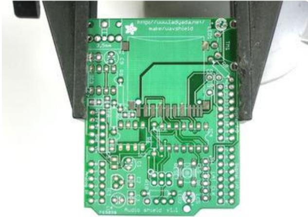
Get ready by placing the PCB in a vise.
