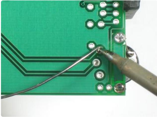
Solder all 5 pins of the potentiometer. Use plenty of solder so that it has a lot of mechanical strength.
