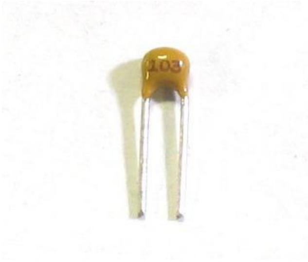
Next is the 0.01uF ceramic capacitor C8. The tricky part here is that in older kits there are many 0.1uF ceramic capacitors in the kit that look identical to the 0.01uF!
