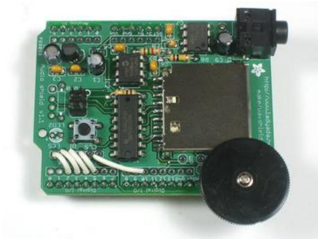
Pins 13, 12 and 11 are used to talk to the SD card and cant be changed. The rest of the pins, however, are more flexible. Still, for all the examples on the site we'll be using this wiring, so it is suggested to just go with this.
