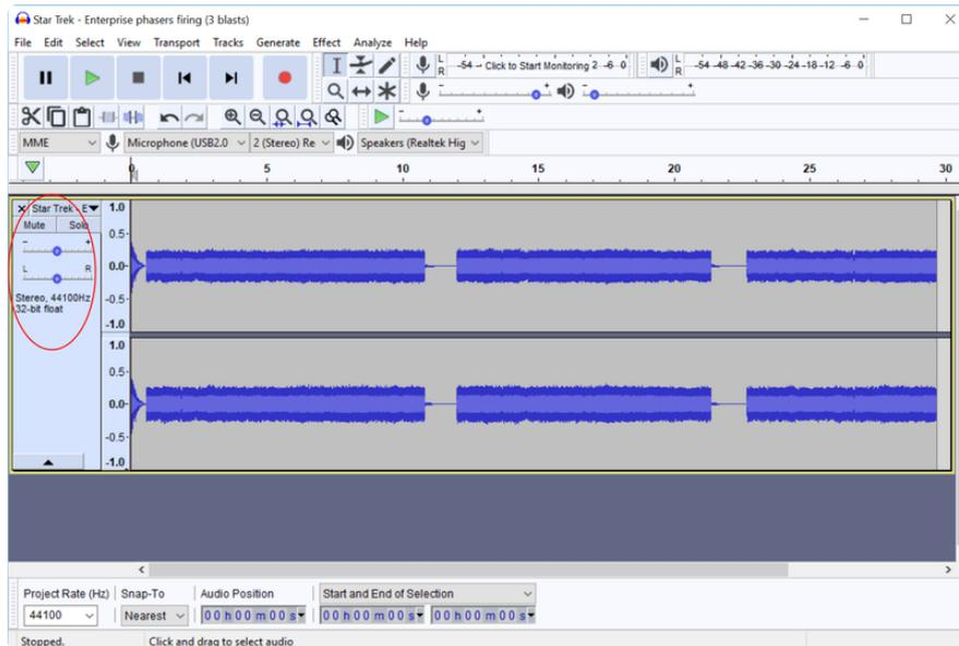
See the red circled text. That shows that the WAV file I chose is a 44.1 KHz, 32 bit stereo file which is above our microcontroller specifications noted (22 KHz, 16 bit, mono). We'll need to tell Audacity what parameters we want to convert the file.
