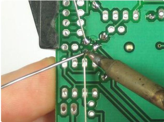
Solder and clip the small capacitor leads.
