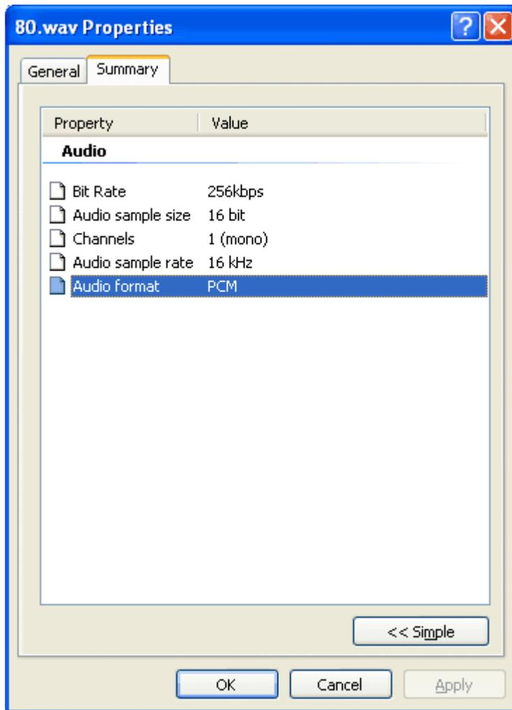
This file is 16KHz, 16-bit, mono PCM. Since that's below the maximum (22KHz, 16-bit, mono PCM) you are good to go. No need to convert the file.
