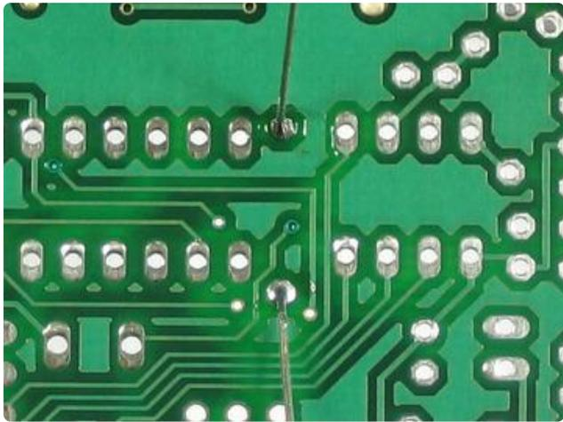
Solder the leads to the pads (metal ring) by heating both with the side-tip of the iron for 3 seconds and then poking in a bit of solder.
