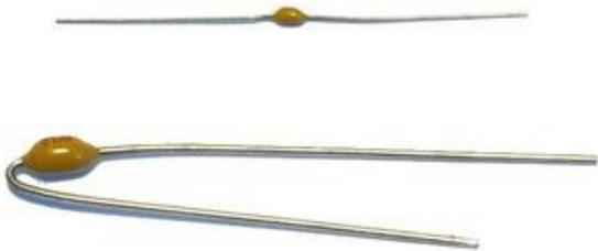
Lately I have been shipping kits with axial (long-ways) package, not radial (side-ways) package. These are longer (see left) and are easy to bend over for soldering. This way there is less confusion. Either way, try to spot the 103 marking.
