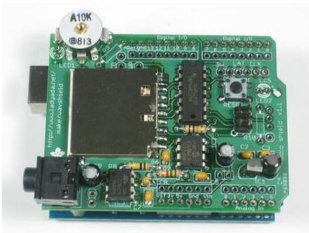
Place the shield PCB onto the arduino so that all the holes match up with the header.
