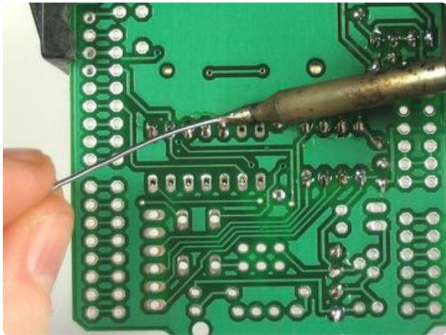
Next is IC4, the buffer to talk to the SD card. Match up the notch just like you did with the smaller chips.
