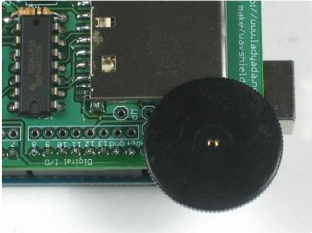
Next you can install the thumbwheel. Use a #0 screwdriver. Align the thumbwheel so it 'grabs' the potentiometer, then gently screw it in place.
