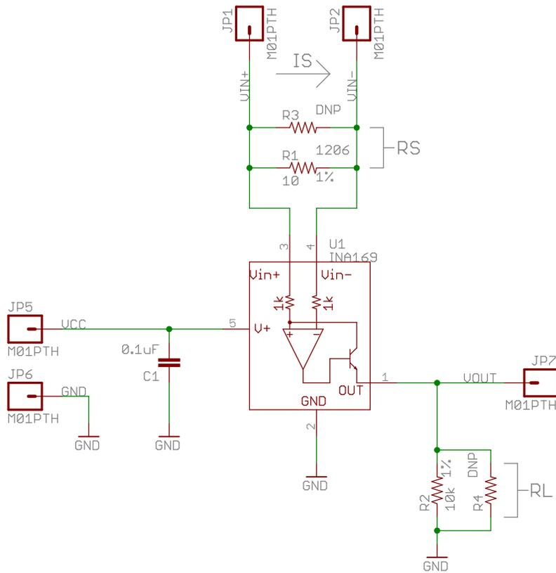
$$V_{OUT} = I_S \times R_S \times R_L / 1k\Omega$$
