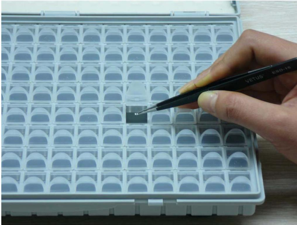
Figure 12. Storing or Obtaining an SMT Component
