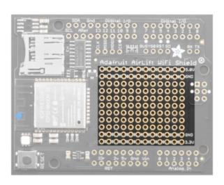
We have a big grid of prototyping holes and power rails if you want to make some custom circuitry!
