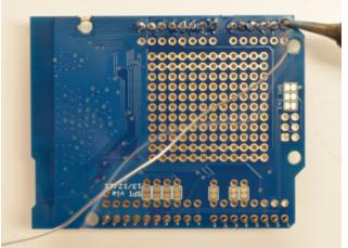
Once you've tacked and straightened all the headers, go back and solder the remaining pins for each header.
