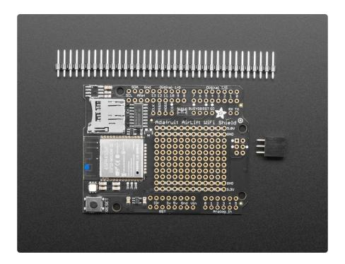
Comes fully assembled and tested, pre-programmed with ESP32 SPI WiFi co-processor firmware that you can use in CircuitPython to use this into WiFi co-processor (). We also include some header so you can solder it in and plug right into your Arduino-compatible, but you can also pick up a set of stacking headers to stack above/below your board.
