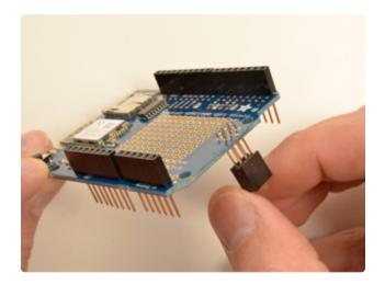
Insert the 2x3 stacking header as shown.
