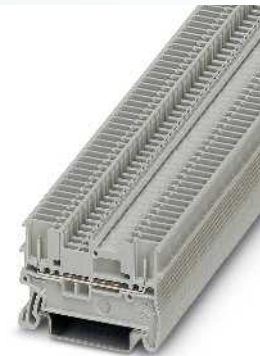
1.5 (1.5) mm 2 , 17.5 A, feed-through terminal block, 2 connections
