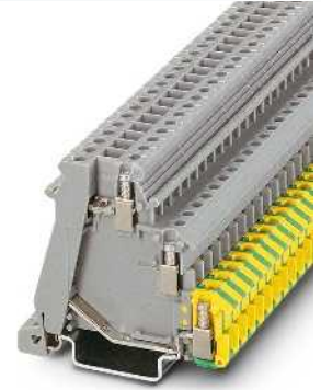
2.5 (4) mm 2 , 26 A, three-conductor actuator terminal block with PE foot
