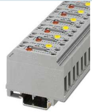
6 (10) mm 2 , 57 A, ground disconnect terminal block
