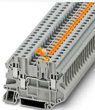
4 (6) mm 2 , 20 A, knife disconnect terminal block, 3 connections
