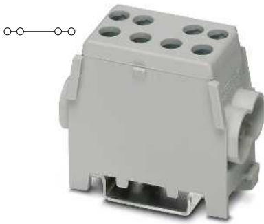
35 (35) mm 2 , 125 A, trunk line branch terminal, 2 x 25 mm 2 feeders
