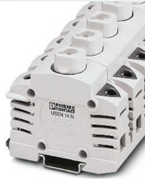
35 (35) mm 2 , 16 A, fuse terminal block for NEOZED D 01 (E14)
