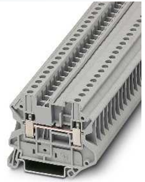
4 (6) mm 2 , 41 A, feed-through terminal block
