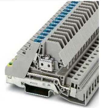
6 (10) mm 2 , 41 A, three-level terminal block, 1 x L phase conductor, 1 x N conductor can be disconnected, 1 x PE
