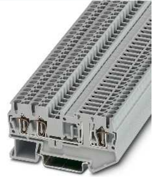
2.5 (4) mm 2 , 20 A, disconnect terminal block, 3 connections
