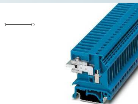
4 (6) mm², 36 A, neutral disconnect terminal block
