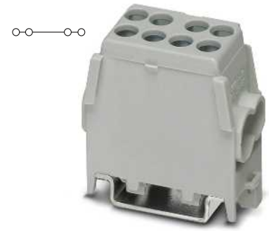
25 (25) mm 2 , 101 A, trunk line branch terminal, 2 x 16 mm 2 feeders
