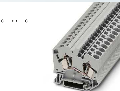
6 (10) mm 2 , 57 A, feed-through terminal block
