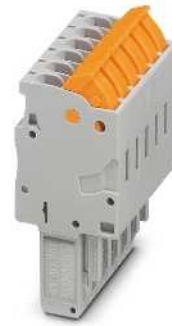
1.5 (1.5) mm 2 , 17.5 A, plug, connection in plug-in direction
