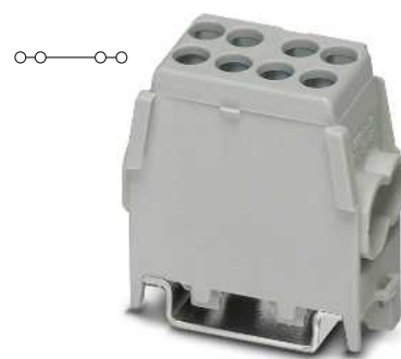
25 (25) mm 2 , 101 A, trunk line branch terminal, 2 x 16 mm 2 feeders
