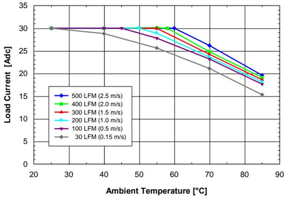
Figure 2: Available output power vs. ambient air temperature and airflow rates for converter DP7130G mounted horizontally with air flowing from pin 1 to pin 22, MOSFET temperature  $\leq 125^\circ\text{C}$ ,  $V_{in} = 12\text{ V}$ .
