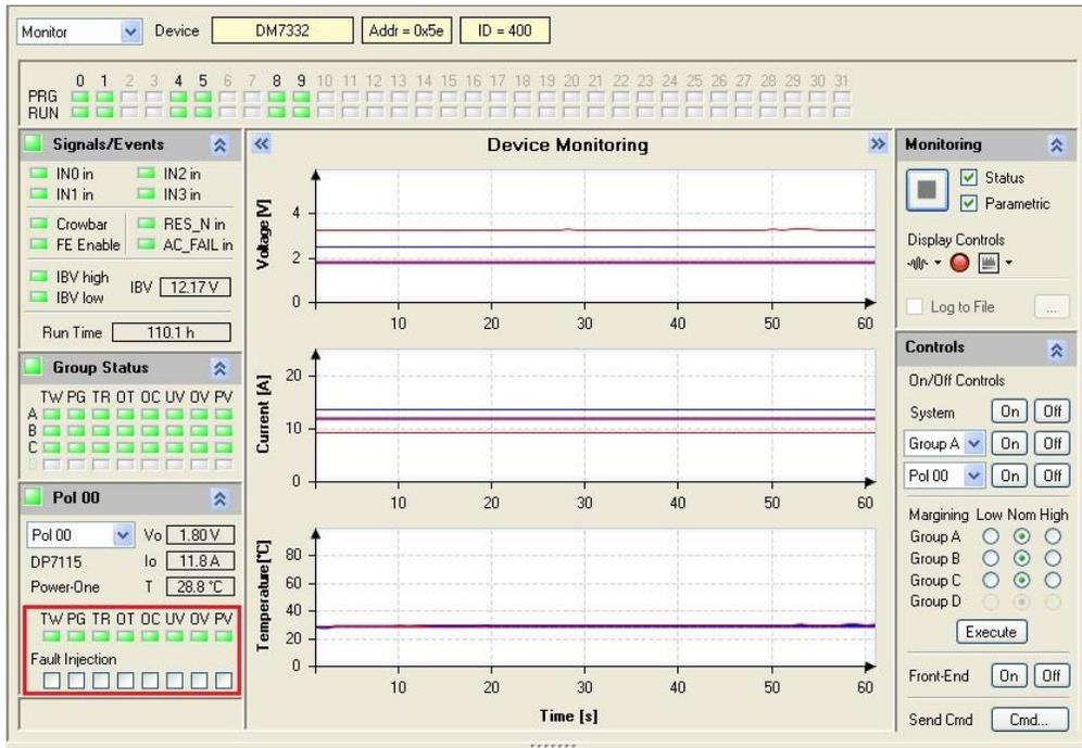
Fault injection into a dPOL requires selecting that dPOL in the POL status dialog in the left column of the Monitoring dialog window. As long as the checkbox is checked, the fault trigger is present in the dPOL. An injected fault is handle by the dPOL in the same fashion as an actual fault. It therefore gets propagated to the other dPOLs / Groups and shuts down in the programmed way the dPOL/Group/System as programmed for that fault.
