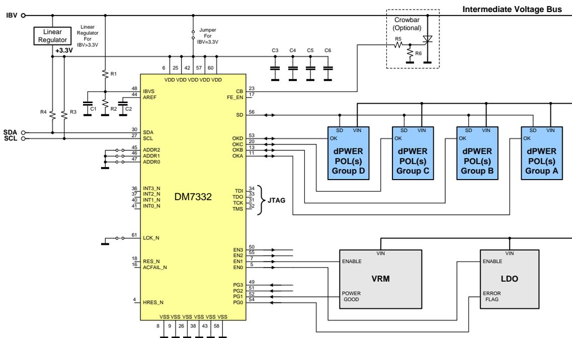
Shown in Figure 54 is a schematic of a typical application of a DP7130G point-of-load converters. The system includes a DM7300 series Digital Power Manager (DPM), at least one DP7130G dPOL, and may include additional DP7130G dPOLs and other d-power® series dPOLs. All dPOLs are connected to the DPM and to each other via a single-wire SD (sync/data) line.
