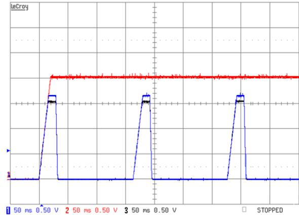
Since both Vo1 and Vo2 have the same delay and slew rate settings they will continue to turn off and on synchronously every 130ms as shown in Figure 38 until the condition causing the undervoltage is removed.
