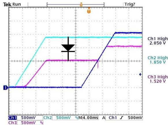
Figure 24 was captured with an actual system where a diode was added to pre-bias a 1.5V bus from a 1.85V bus in order to simulate the effect of current leakage through protection circuits of unpowered logic connected to powered logic outputs (a common source of pre-bias in power systems).
