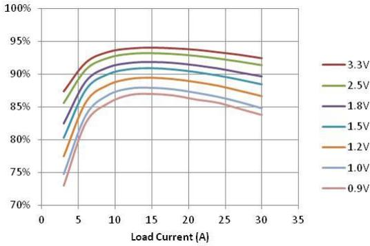
Figure 6: Efficiency vs. load current and input voltage for converter DP7130G at 12V in, Ta = 25 °C.
