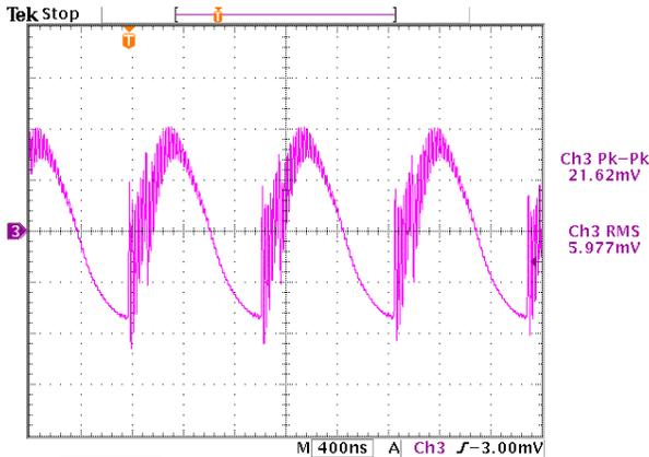
Figure 45. Output Voltage Noise, Full Load, 180° Interleave
