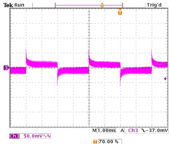
As noted earlier, increasing the Load Regulation parameter provides load dependant dynamic load positioning. This shows up in the following figure.
