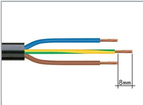
1. Strip length, outer insulation = 30 mm (2-pole), 37 mm (3-pole), 45 mm (4- and 5-pole)
