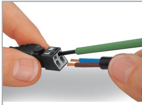
To terminate fine-stranded conductors, open the clamping unit via screwdriver – 2.5 mm blade width – and insert a stripped conductor until it hits the backstop. Terminate solid conductors by simply pushing them in.
