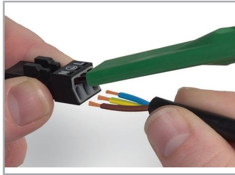
To terminate fine-stranded conductors, open clamping units via operating tool (890-382) and insert stripped conductors until they hit backstop.
