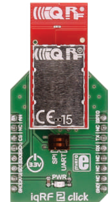
iQRF 2 Click With DCTR-72DAT RF transceiver, operating in the 868/916 MHz frequency.
