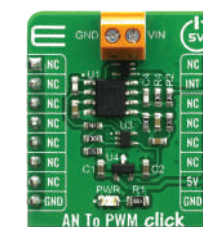
AN To PWM click Uses OPA365 series op-amps, and the TLV3201 comparators from TI.
