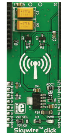
Skywire™ Click Adapter Click, which hosts NimbeLink/Skywire™ cellular modems [using stacking headers]. MSRP - $19 00 MIKROE-2405
