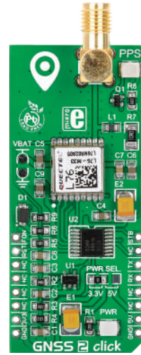
GNSS 2 Click Quectel's L76 module and SMA antenna with an external antenna connector. GPS + GLONASS.
