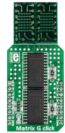
Matrix G Click Matrix text display with two green 5x7 matrices and two MAX7219 8-bit LED drivers. MSRP - $29 00 MIKROE-2246
