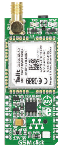
GSM Click With quad-band GL865-QUAD GSM/GPRS module, onboard antenna connector and SIM card socket.
