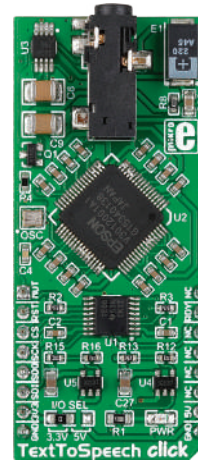
TextToSpeech Click With S1V30120 speech synthesis IC powered by the Fonix DECTalk® v5 speech synthesis engine.
