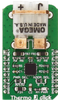
Thermo J Click It is a temperature measurement Click board™, which uses a thermocouple type-J probe. MSRP - $24 00 MIKROE-2811
