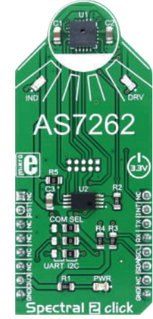
Spectral 2 Click Uses the AS7262, 6 channel visible spectral_ID device with electronic shutter and smart Interface.
