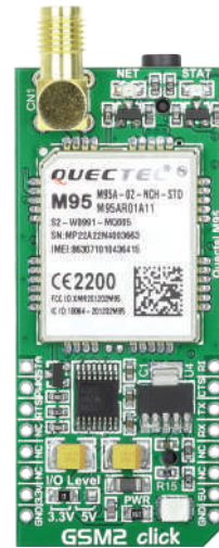
GSM 2 Click With Quectel's M95 FA quad-band GSM/GPRS module. 85.6 kbps GPRS data transfer.
