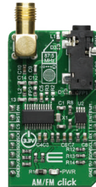
AM/FM Click Based on the Si4731 IC - digital CMOS AM/FM radio receiver from Silicon Labs.
