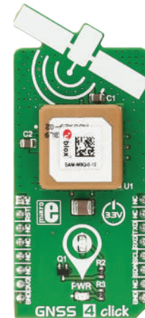
GNSS 4 Click It features SAM-M8Q patch antenna module from u-blox.
