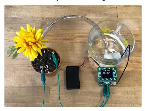
It's easy to use the Adafruit Bonsai Buckaroo with CircuitPython. This example uses the <u>Adafruit CircuitPython CLUE</u> () library to display soil moisture level and the status of the pump motor on the CLUE display. Connect your Bonsai Buckaroo to your CLUE, and connect the motor and plant to the Bonsai Buckaroo, and you're on your way to automatic plant care. Let's take a look!
