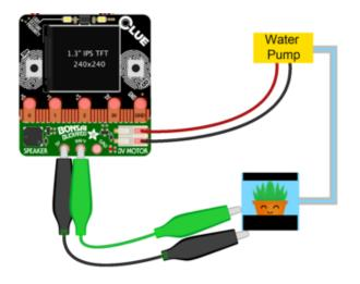
Mount the Bonsai Buckaroo to the CLUE using the included mounting hardware. Connect the red wire of the water pump to the top of the motor controller terminal. Connect the black wire of the water pump to the bottom of the motor controller terminal.
