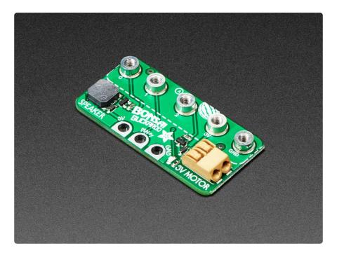
We can't wait for spring to arrive, and we're looking forward to caring for some plants! We designed this little add-on for <a href="micro:bit">micro:bit</a> ()or <a href="CLUE">CLUE</a> () boards – bolt it on with 5 screws to get a buzzer/beeper, motor driver, and breakouts for connecting a <a href="mailto:soil">soil</a> sensor () (two alligator clips + nails work just fine). Simple, but effective!
