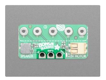
In the center are the Alligator clip pads for pin P1, 3V and GND. Connect to two alligator clips and nails to measure soil resistance as shown on the next pages
