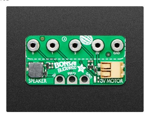
The Bonsai Buckaroo is designed to add a speaker, motor terminal, and pins for connecting a soil sensor to your micro:bit or CLUE board. Let's take a look!
