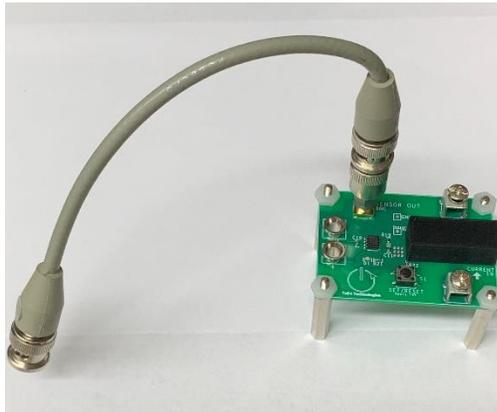
Figure 3: SMA-to-BNC with Short BNC Cable
