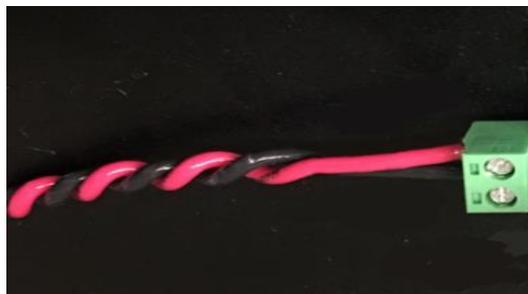
Figure 2: Example of Twisted Leads for Voltage Supply
