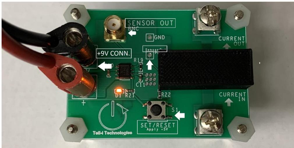
Figure 1: Connections and Reference of Evaluation Board w/ DS10.2S Current Sensor
