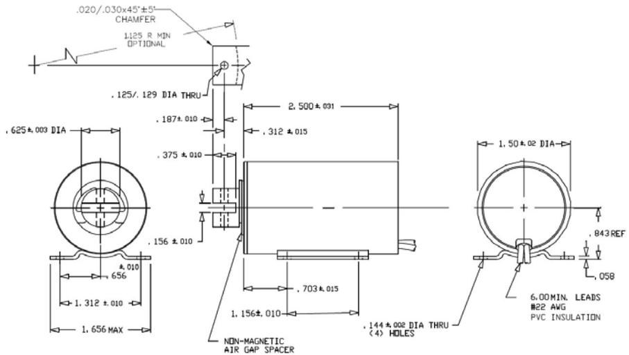
Solenoid shown energized with plunger fully seated
