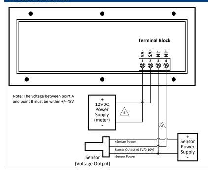
This example illustrates an application where the voltage output sensor is connected to terminals 3 and 4, where terminal 3 is the negative input terminal (-IN) and terminal 4 is the positive input terminal (+IN).
