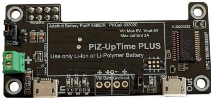
All operating parameters are customized using the sample Python script. These are communicated from the Pi to the PiZ-UpTime PLUS via I<sup>2</sup>C, usually during the reboot. Different operating modes supported are:
