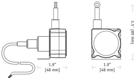
The SP3 from Celesco is a compact, economical stringpot that provides a user selectable 4-20 mA or 0-10 Vdc output signal. Simply install this sensor using the handy mounting bracket and connect the appropriate wires for the desired output.
