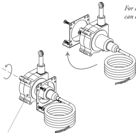
To change measuring cable direction simply remove the 3 bracket attaching screws and rotate sensor body to desired direction.
