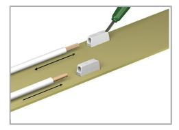
Insert fine-stranded conductors and remove all conductor types via operating tool. Solid conductors can also be terminated by simply pushing them in.
