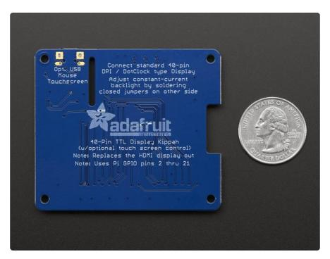
Comes as one fully assembled and tested DPI Kippah circuit board. You may need a soldering iron to adjust the backlight by soldering closed a PCB jumper (check the tutorial on this). TFT display (), USB micro-B cable (http://adafru.it/592), FPC extension
