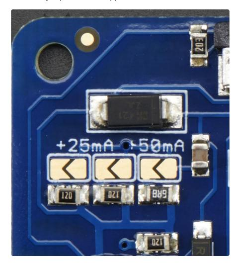
The left and middle jumper each add 25mA to the default 25mA. The right jumper adds 50mA. So if you want to have a 50mA backlight, short only the left jumper. For 75mA, short the right most. For 100mA solder short the left and right and for 125mA short all three!
