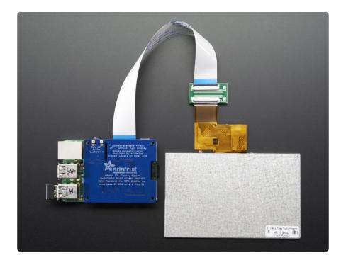
Check the Downloads page for an example datasheet so you can check if your display is compatible. All Adafruit 40-pin TFT TTL displays work, we do not guarantee any other displays work.
