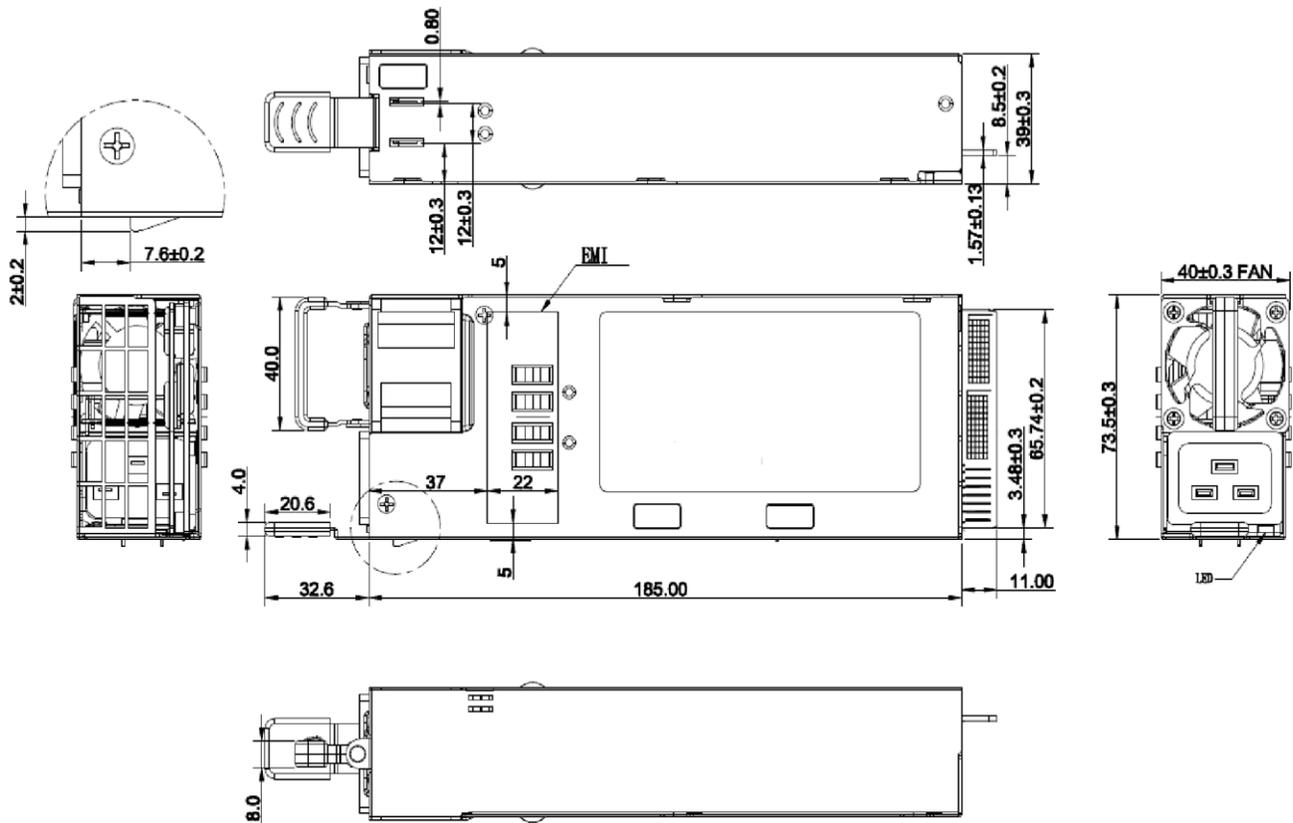
Figure 18. Mechanical Drawing
