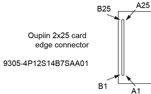
Figure 19. Back DC output golden finger port
