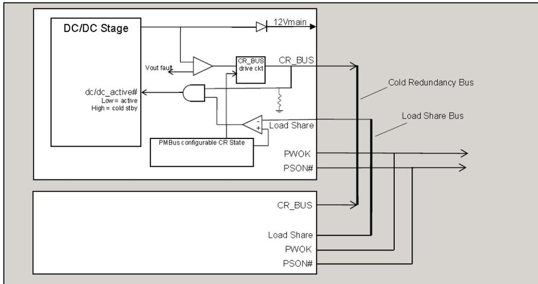
Figure 15. Cold Redundancy 1+1 Functional Block Diagram
