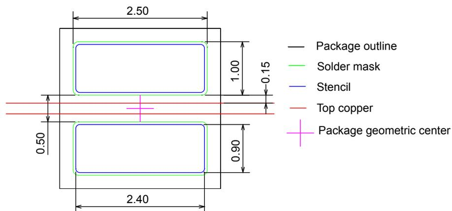
Figure 3. Recommended PCB footprint design for the LUXEON emitter. Dimensions are in mm.
