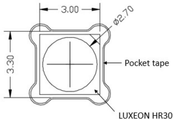
Figure 9. LUXEON emitter in a pocket tape. Dimensions in mm. Best to use nozzle with outer diameter between 2.7mm and 3.3mm to avoid interfering with the pocket tape cavity or picking solely from the silicones.
