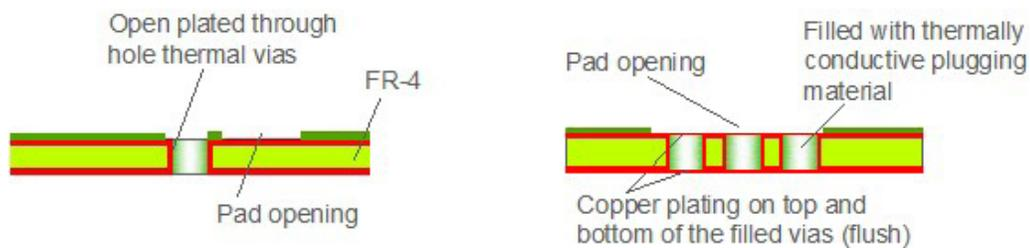
Figure 5. Left picture shows a cross section of an open via with plated through hole design with one pad opening where the LED pad is soldered onto. Right picture shows a cross section of a filled and cap via design with one pad opening. One of the LED pads is then soldered on top of the flush area where the filled and capped vias are underneath it to create direct thermal path connection between LED and bottom of PCB.
