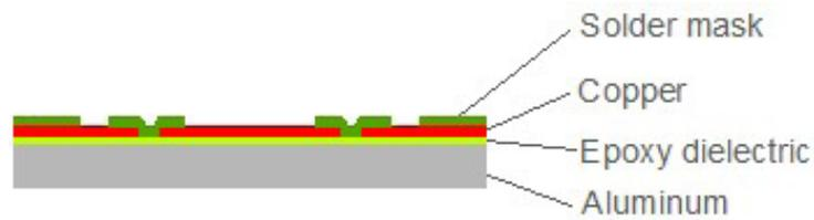
**Figure 4. MCPCB typical cross section of the three-pad openings with aluminum substrate.**
