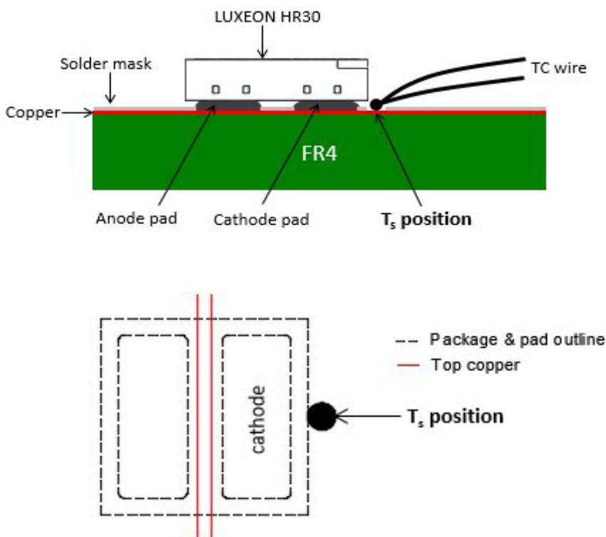
Figure 7. The recommended temperature measurement point  $T_s$  is located on the cathode copper layer of the PCB, closest to the package. The top picture shows the side view. Bottom picture shows the top view of the  $T_s$  location.
