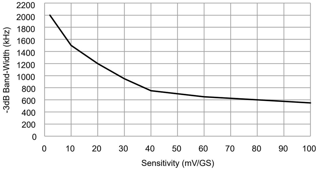
Figure 4. Sensitivity VS Band-width
