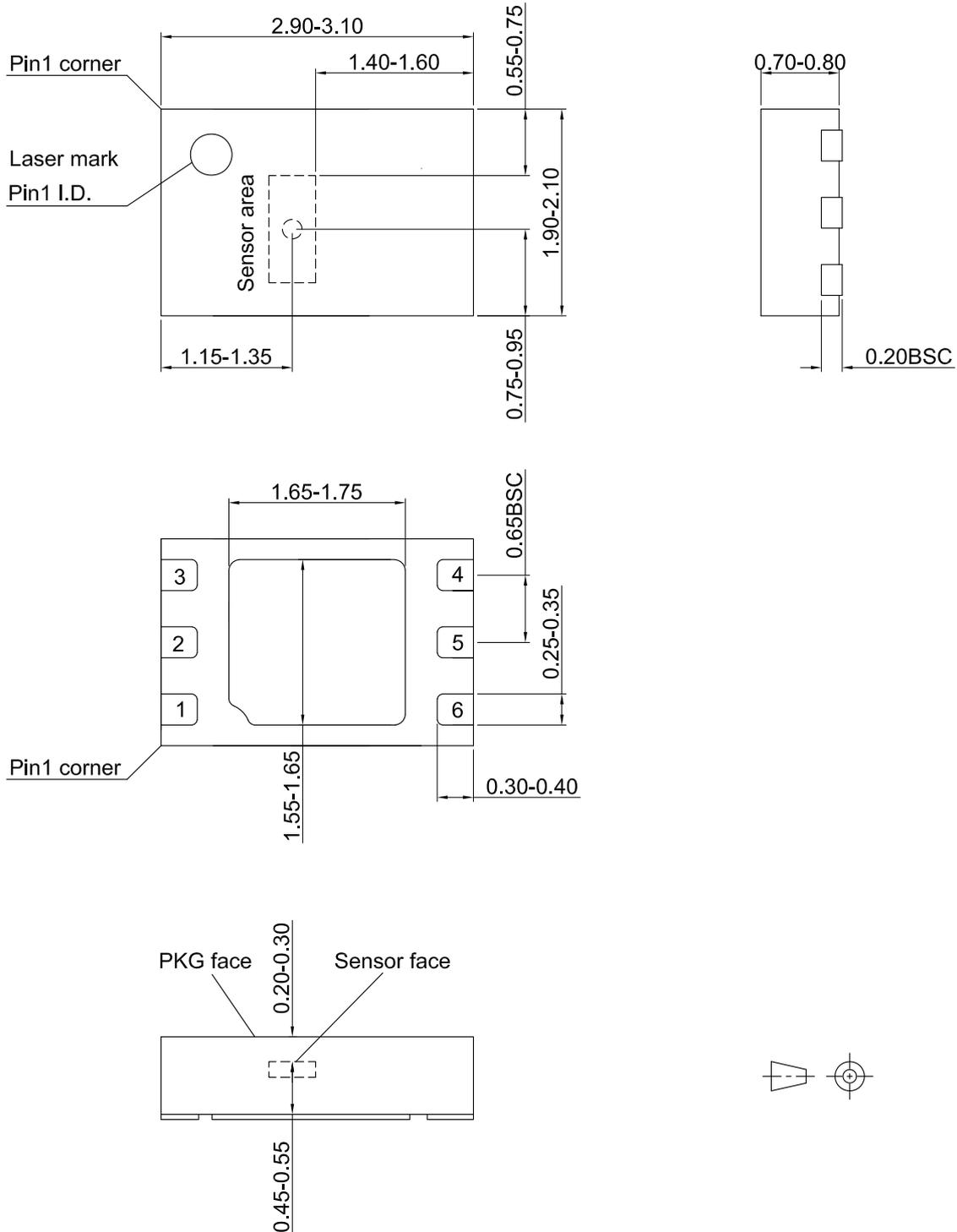
Figure 6. Package outline of DFN6L (unit: mm)
