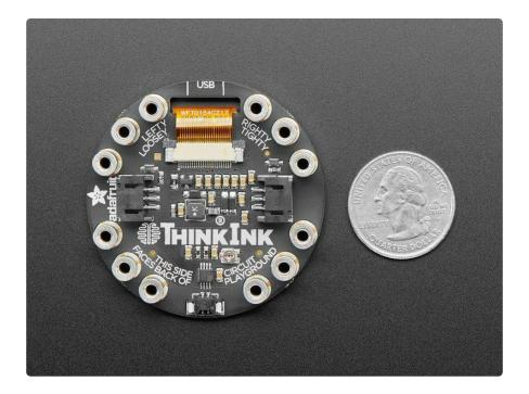
Once attached you'll get a 1.54" 152x152 display (black and red ink pixels and a whiteish background), two 3-pin STEMMA connectors for <u>attaching NeoPixel strips</u> () or <u>serv</u> os (), and a Class D audio amplifier with <u>a Molex PicoBlade connector that can plug</u> one of our lil speakers ().
