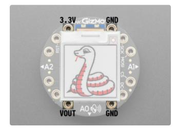
VOUT - power input, connect to 3-5VDC. GND - power and signal ground. Connect to your power supply and microcontroller ground.
