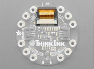
Front and center is a 1.54" 152x152 tri-color e-ink display, with black and red ink pixels and a white-ish background. The display cable goes through to the back and connects to the display connector towards the top in the middle of the back.
