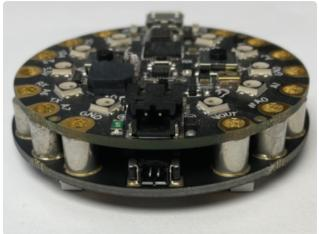
Place the Circuit Playground board on top of the Gizmo being sure that the connectors mentioned in the previous step are still aligned.
