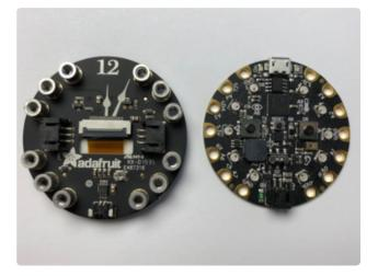
Start by aligning the two boards side by side like in the photo with the black plastic speaker connector and battery connectors pointing in the same direction.
