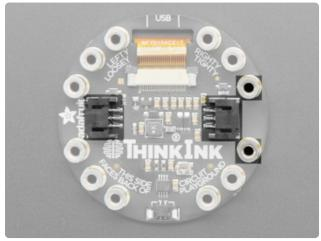
On the sides of the back are two 3-pin STEMMA connectors for hooking up NeoPixels or servos connected to pins A1 and A2.
