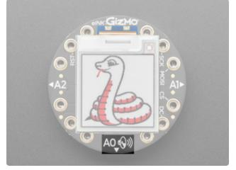
On the bottom of the back, there is a Molex Picoblade speaker connector and a class D amplifier connected to pin A0. The location is labeled on the front as A0 with a speaker symbol.
