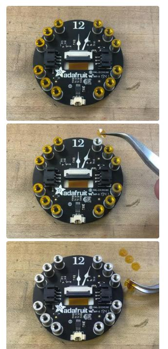
The amber colored Kapton tape dots must be removed from each of the twelve standoffs before assembling the boards. These are electrically insulating and will prevent the Gizmo from working properly if left in place.
