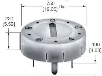
screwdriver/coin actuated Part Number 435005-1
