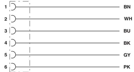
Contact assignment of M8 socket
