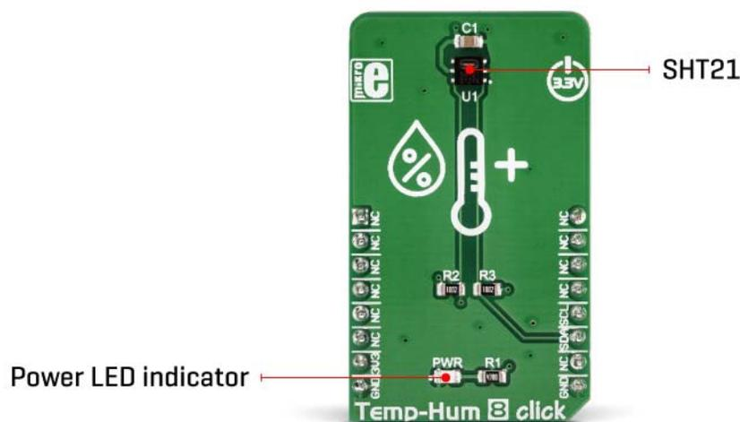
The SHT21 IC is based on the CMOSens® technology, featuring the capacitive RH sensor and the bandgap temperature sensor. Besides the sensing elements, the IC incorporates an analog front end (AFE), which consists of A/D converter, OTP memory, and a logic section. The integrated
