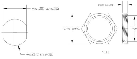
NOTE: MATERIAL HOUSING: PBT UL94V-0, BLACK CONTACT: BRASS NUT: STAINLESS STEEL 316 SHELL: STAINLESS STEEL 316 D-RING: EPDM, BLACK FINISH CONTACT: UNDER PLATE: ELECTRICAL RATED CURRENT: RATED VOLTAGE:
