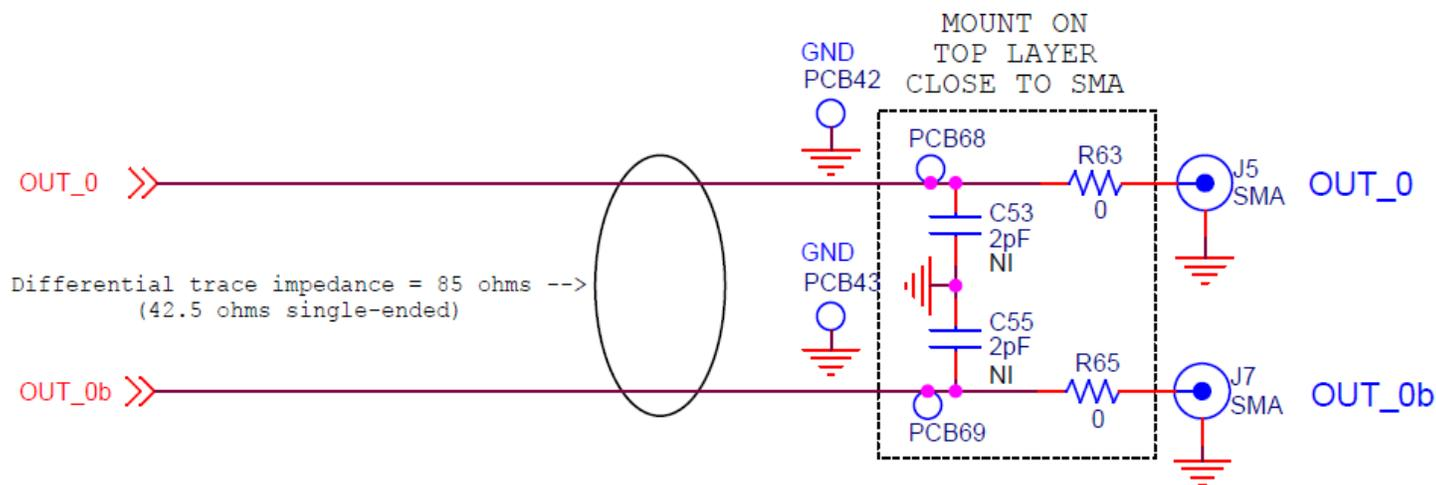
Figure 4.1. Si53258-EVB Output Clock Differential Pair Termination Circuit
