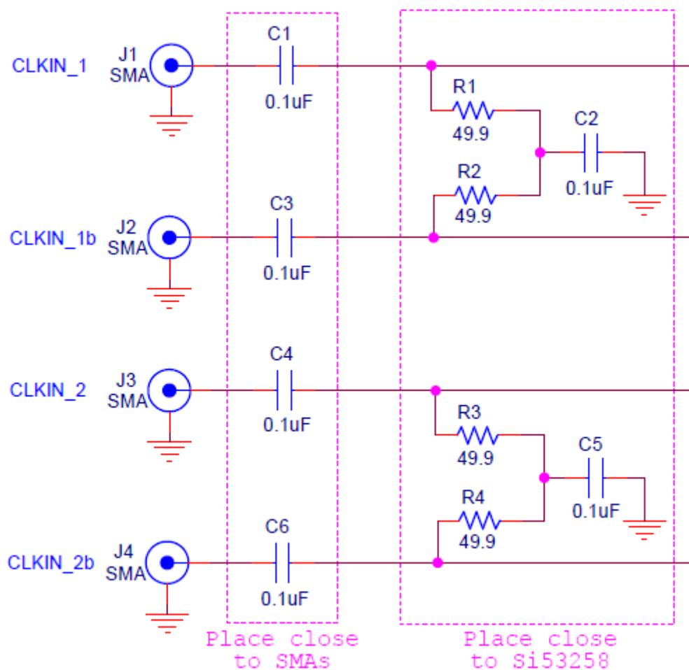
Figure 5.1. Si53258-EVB Input Clock Differential Pair Termination Circuit
