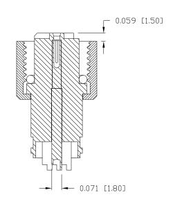
MATERIAL HOUSING: TPU UL94V-0, BLACK CONTACT: BRASS NUT: BRASS **EPDM** □-RING: FINISH CONTACT: GOLD PLATED OVER 50u" NICKEL NICKEL PLATED NUT: ELECTRICAL RATED CURRENT: 4A RATED VOLTAGE: 250V INSULATION RESISTANCE: 100 MOhms MIN. 10 mOhms MAX. CONTACT RESISTANCE: WATER PROOF: IP67 ENVIRONMENT OPERATION TEMPERATURE: -40°C TD +85°C
